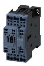
power contactor, AC-3e/AC-3, 9 A, 4 kW / 400 V, 3-pole, 24 V DC, auxiliary contacts: 1 NO + 1 NC, spring-loaded terminal, size: S0, communication-capable
