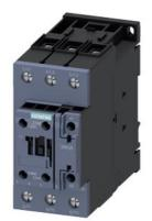
power contactor, AC-3e/AC-3, 65 A, 30 kW / 400 V, 3-pole, 24 V DC, 0.8-1.2\* Us, with integrated varistor, auxiliary contacts: 1 NO + 1 NC, screw terminal, size: S2, suitable for PLC outputs
