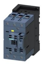
power contactor, AC-3e/AC-3, 80 A, 37 kW / 400 V, 3-pole, 175-280 V AC/DC, 50/60 Hz, with integrated varistor, auxiliary contacts: 1 NC, main circuit: screw terminal, control and auxiliary circuit: spring-loaded terminal, size: S3, F-PLC-IN
