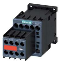
contactor relay, 6 NO + 2 NC, 230 V AC, 50/60 Hz, screw terminal, frame size S00, captive auxiliary switch
